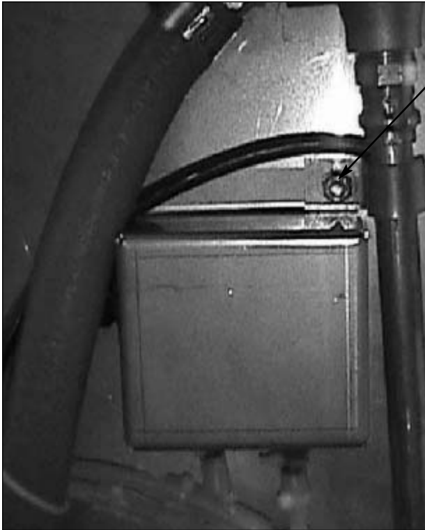
Back of machine showing use of existing mounting hardware for installation of vacuum switch assembly.
